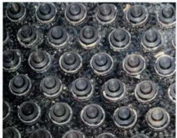
Studs are installed in a matrix pattern
